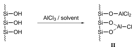
Scheme 7 Preparation of supported aluminium chloride
